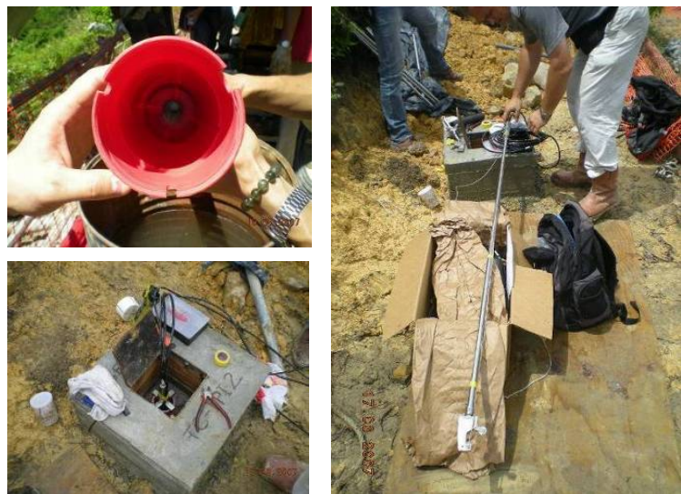
Fig. 13b. Inclinometer monitoring system (Millis et al. , 2008)
