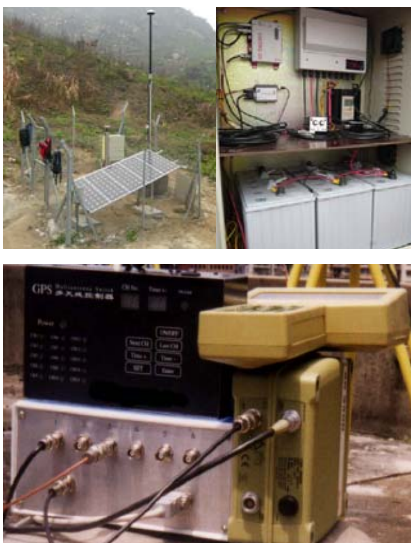
Fig. 13a. DGPS (top) monitoring equipment and (bottom) multi-antenna system (Millis et al. , 2008)
