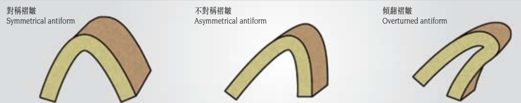
圖7-6d. 褶皺的種類。 Figure 7-6d. Types of folds.
