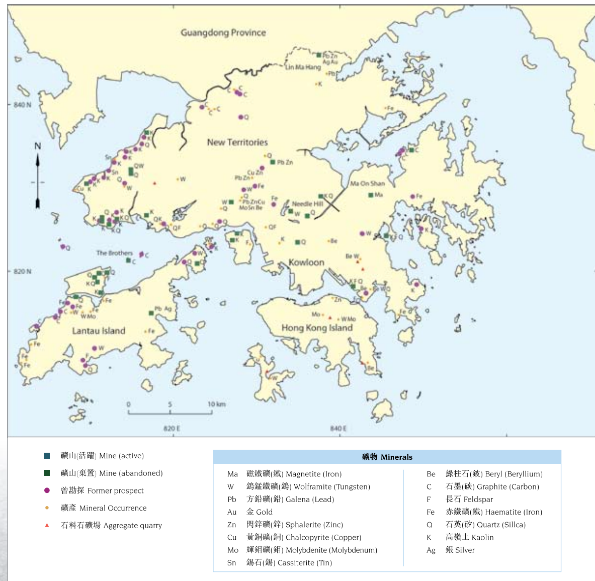
圖8-1. 香港具經濟價值的礦產位置圖。 Figure 8-1. Location of economic mineral occurrences in Hong Kong.
