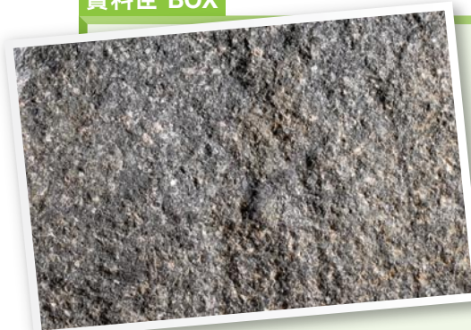
圖1-14. 粗火山灰晶屑凝灰岩，主要含有晶體碎屑。 Figure 1-14. Coarse ash crystal tuff, containing mainly crystal fragments.
