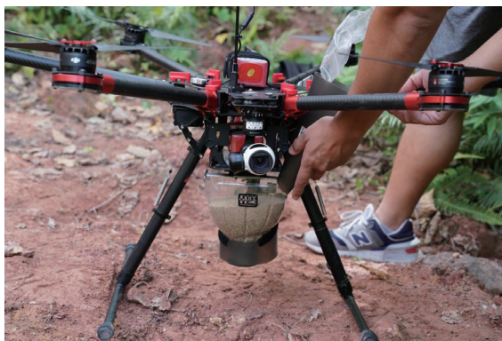
↑ 無人機裝有自行開發的播種器，配合香港的情況。(The drone is equipped with a seeder developed specifically for Hong Kong's environment.)
