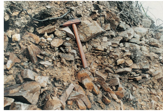
圖10. 在天然山坡上常見受侵蝕的岩石碎屑層(坡積物)。 Figure 10. A layer of eroded debris (colluvium) is common on most natural hillsides.
