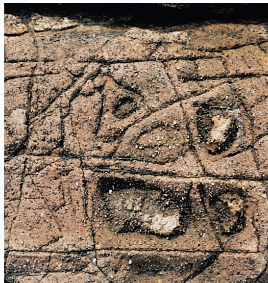
圖3. 火山岩受到不均勻的風化，突顯其節理及成份。 Figure 3. Differential weathering of a volcanic rock, emphasising the joint pattern and components.
