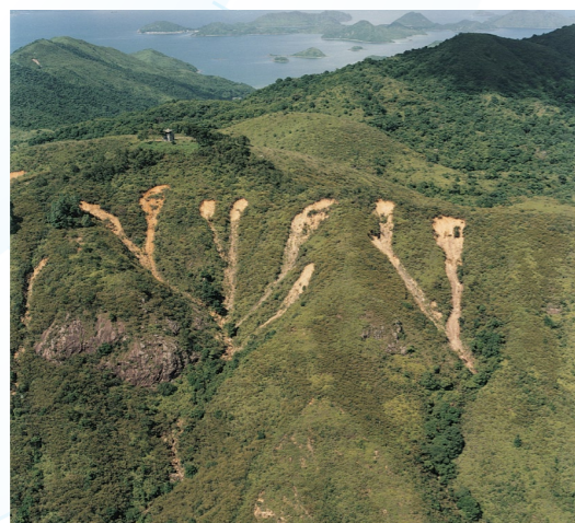
圖12. 由淺層滑坡聚合而成的沿溝泥石流崩塌。 Figure 12. Coalescing channelised debris avalanches originating from shallow failure scars.
