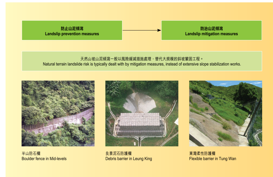
圖38. 一些防治天然山坡山泥傾瀉的風險緩減措施例子。 Figure 38. Some examples of natural terrain landslide mitigation measures.
