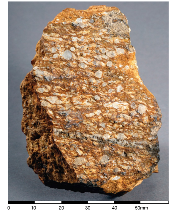
圖15. 片岩一為有葉理變質岩的例子。 Figure 15. Schist - an example of foliated metamorphic rock.
