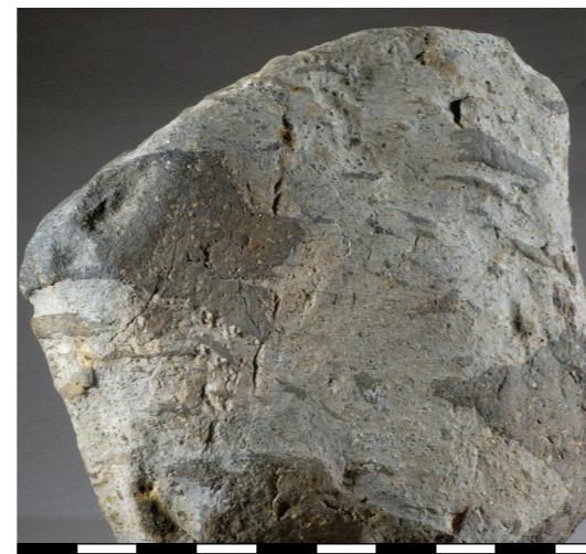
圖6. 條紋斑狀凝灰岩(熔結凝灰岩)，含有在其形成時被壓扁的浮石碎塊(火焰石)及玻璃碎片。 Figure 6. Eutaxitic tuff (welded tuff), containing pumice fragments (fiamme) and glass shards that are flattened during its formation.
