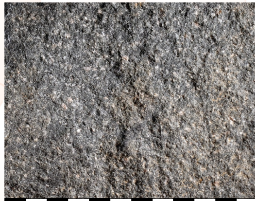
圖5. 粗火山灰晶屑凝灰岩，主要含有晶體碎屑。 Figure 5. Coarse ash crystal tuff, containing mainly crystal fragments.
