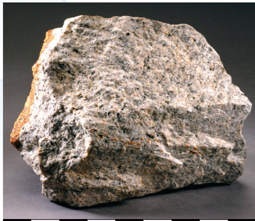
圖18. 斑狀細粒花崗岩(晚侏羅紀針山花崗岩)。 Figure 18. Porphyritic fine-grained granite (Late Jurassic Needle Hill Granite).
