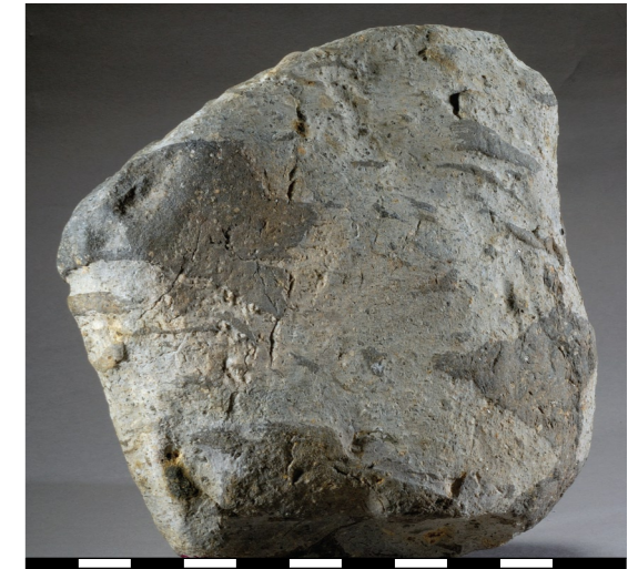
圖12. 早白堊紀淺水灣火山岩群的條紋斑狀細火山灰玻屑凝灰岩。 Figure 12. Eutaxitic fine ash vitric tuff of the Early Cretaceous Repulse Bay Volcanic Group.
